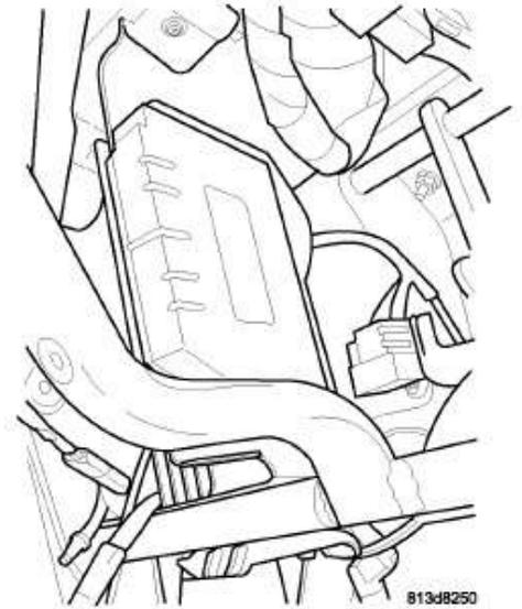
Access is obtained by removing the lower kick panel (has deck lid release button) and cover below the steering wheel and instrument cluster.
