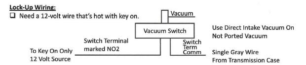
The switch is adjustable from 6" to 22" of vacuum. Turning the screw clockwise will make the trigger point happen sooner as the vacuum drops. (Roughly 6" at max turns in.) Turning the screw counterclockwise will push the trigger point back until a lower vacuum is achieved. (Roughly 1" at max turns out.) If your vehicle surges in and out of lock-up, please turn the vacuum switch adjustment screw 2 turns counterclockwise.
